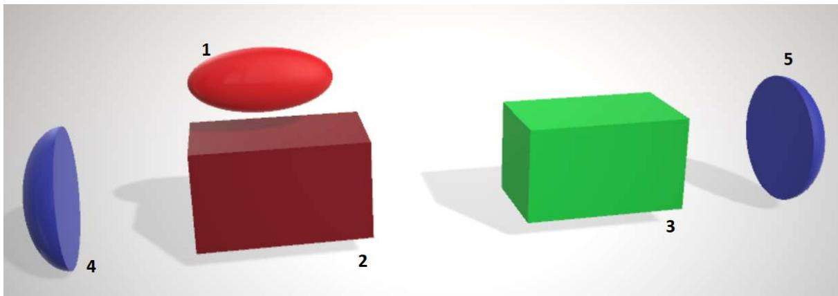
Fig 1. Basic layout of a DPSS laser
