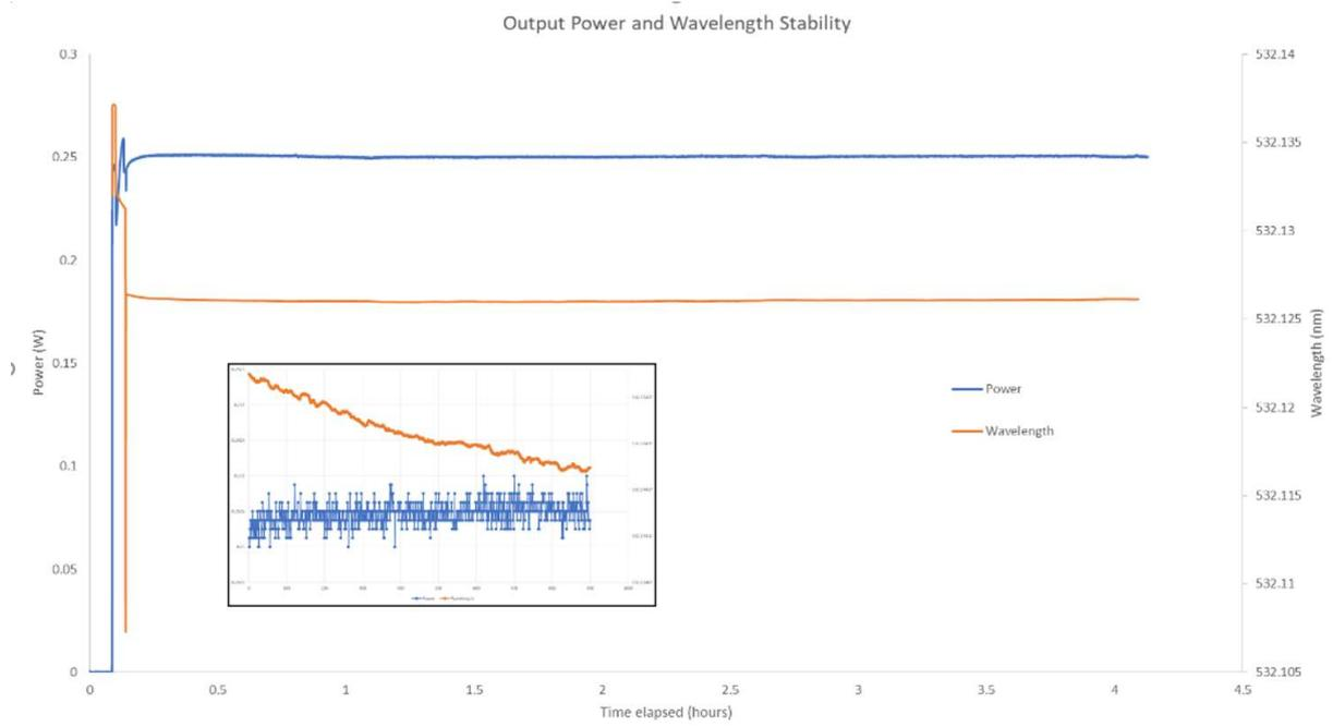
Fig 10. Data taken with a 250 mw Solo-640 on an optical bench over 4 hours.
